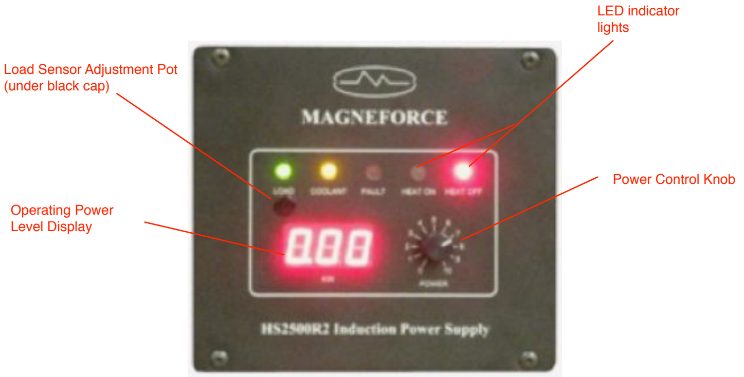
HS2500R2 Standard Control Panel
