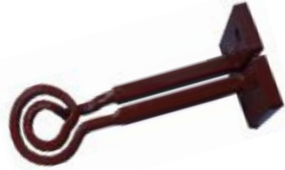
A 2 turn flat pancake type coil for heating an isolated spot on a steel strip. Insulated with red epoxy powder coat.
