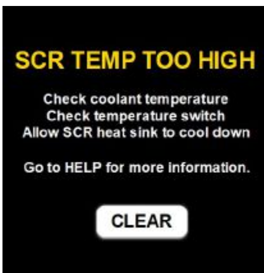
Figure 48. SCR Temp TOO HIGH Warning Screen
