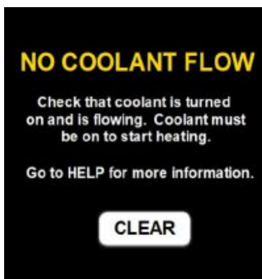
Figure 47. No Coolant Warning Screen
