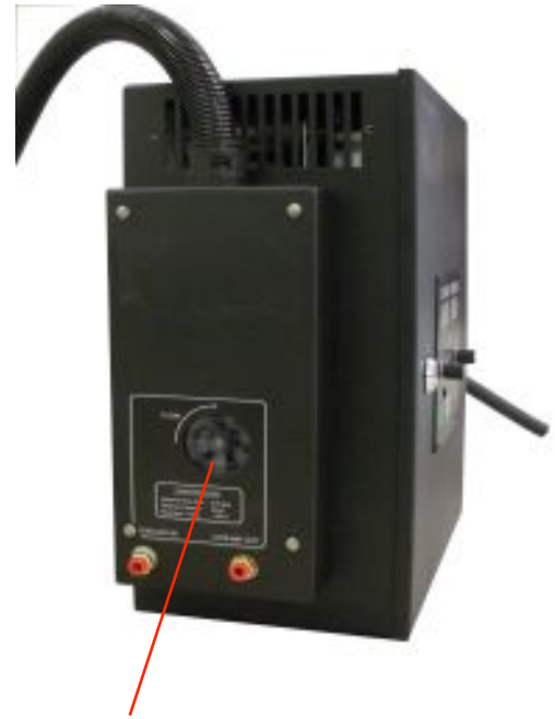
Coolant Flow Paddlewheel must turn clockwise
