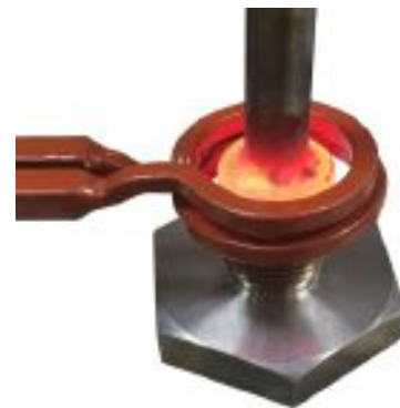
A fitting is brazed to a pipe with a solenoid coil
