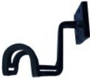
A "C" shaped coil allows a section of a long shaft to be easily inserted in the coil for a carbide insert brazing application. Coil head is plasma sprayed ceramic.
