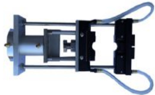
Pneumatically operated split coil for soldering a large fitting to a coaxial cable. The two halves of the coil open and close to allow insertion of the fitting and to provide even heat around the circular connector body.
